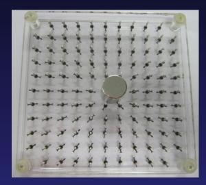
North poles attract South poles and repel other North poles. If you turn the magnet so that the other face is closer to the magnetic model field, you should see the arrows reverse their previous direction. The side of the magnets that was attracted to the first magnetic pole is now repelled, the end of the magnetic arrows that was repelled is now attracted. Moving the magnet around, the magnetic arrows will follow the magnet.
